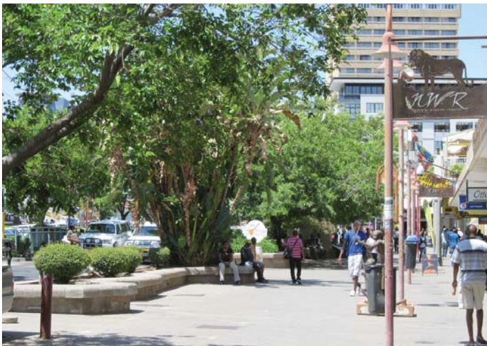
Figure 32 Street furniture providing vehicle and pedestrian buffer
